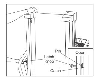
Hold the treadmill firmly with both hands, and lower the treadmill to the floor. Do not drop the treadmill frame to the floor. CAUTION: To decrease the possibility of injury, bend your legs and keep your back straight.
